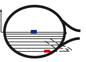
Insert the end of the string into the holes at the knot. There are usually 2 located in the crease of the racket. Only if the string cannot pass, special hooks can be used to widen the opening. Be careful not to damage the string that is already in the hole.
