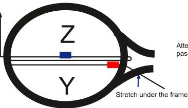
Attention! The strings that come out of the holes in the middle must pass under the frame to avoid unwanted deformation during the pull.
