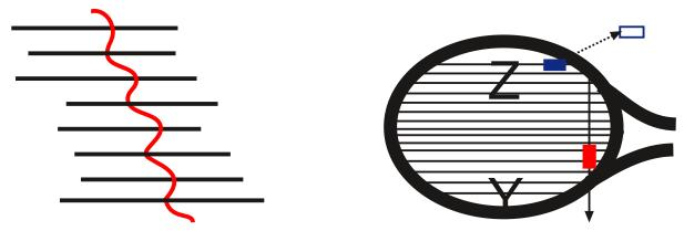
After you zig zag over the string, pull it with the counterweight arm, release the Z pliers and fix the string just stretched with the Y pliers from the Y side. Now use both pliers, relatively halfway between them, to fix the stretched strings.
