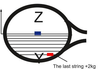
Attention! Try to place the pliers close to the racket frame. Pay special attention when weaving the last vertical string from the Y side. It must be pulled with a load 2kg higher than the tension of the other strings. This is because you will then end the string with a knot and there will be a natural loss of string tension. Use the node function (N1). After stretching the string, fix it with Y pliers and make a closing knot.
