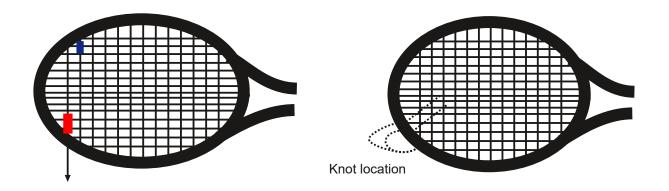
The string pattern is closed. Now release the string with the pliers and remove the racket from the fixation.
