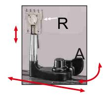
With these pliers, we can reach all places inside the racket and can attach the strings both vertically and horizontally.
