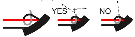
If you don't have special pliers, you can also twist the string on a piece of round wood (while doing so, you must make sure that the string does not get tangled). We recommend making two knots in a row on one string, one opposite the other. After closing the knot, release the Y pliers, which will not be used for a while.
