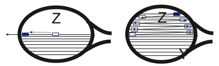
ATTENTION! After closing all the vertical strings, we recommend checking the 6 clamps that fix the racket. The racket is under concentric thrust, so it is necessary to adjust the fixation to changes in the shape of the racket.
