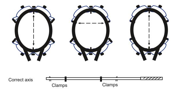
ATTENTION: Check that the frame is correctly aligned. In case of misalignment, damage and deformation or cracks may occur!
